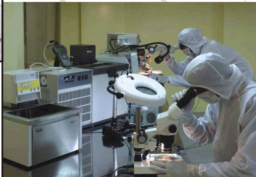
Chip Bonding in Class 100K Clean Room
